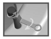
Screw the nut clockwise to separate it from the sensor by wrench and then screw out the sensor by hand
