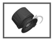
Or disassemble the case of the sensor by the bottom cover if the wrench is lost
