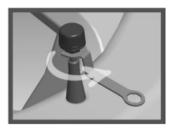
Tighten the nut anticlockwise by wrench
