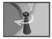
Screw the nuts to the bottom of the valve core
